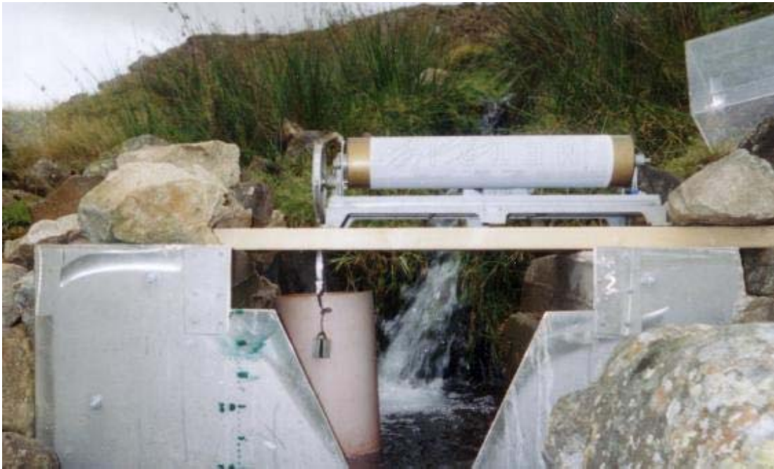
Figure 4.3.b, a photo showing the chart recorder installed at the weir.
