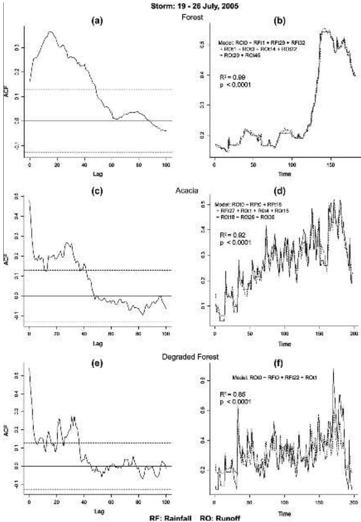
**Fig. 10.** Coastal basins: The cross-correlation coefficients and time series-regression models (Eq. (2)) for the Forest (NF1), Acacia (AC1) and Degraded Forest (DF1) for the Event 3 (19–26 July 2005). Note: 1 lag unit is equal to 0.6 h and the time is expressed in lag units.
