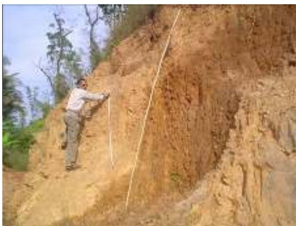
**Fig. 2.** A deeply weathered Red soil profile which is located near the Malnaad (Kodigibail) basins. The depth of the soil profile is in excess of 2 m depth and preferential wetting is also evident. Weathered rock is also visible in the right bottom corner.
