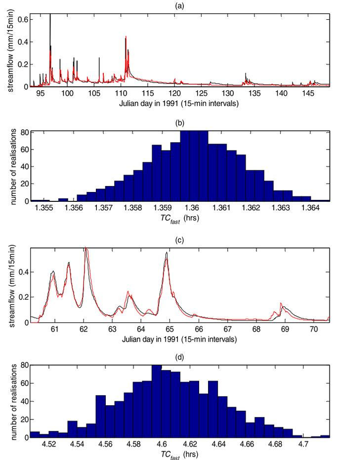
**Fig. 3.** Example observations and model results for period 4 (a tropical basin) and 11 (a temperate basin) shown in Table 1. (a) and (c) Observed (—) and simulated streamflow (—) for periods 4 and 11, respectively. (b) and (d) Frequency distribution of the Dynamic Response Characteristic of the  $TC_{fast}$  for periods 4 and 11, respectively, estimated using uncertainty information implicit to the RIVC method applied in 1000 Monte Carlo realizations.
