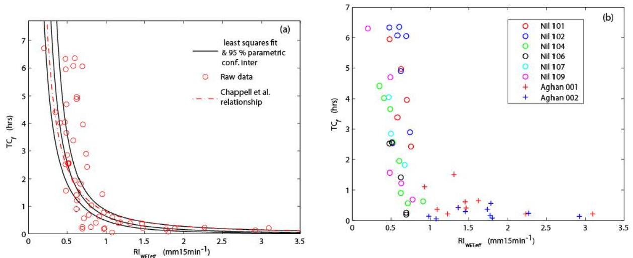
Figure 3-4: The relationship between the fast component of storm hydrograph flashiness ( $TC_f$ ) and average rainstorm intensity based in 15-minute periods with rainfall ( $RI_{WETeff}$ ), where (a) shows the trend and its uncertainty (and consistency with Chappell et al., 2017 trend), while (b) shows the catchments utilised in the relationship, where ‘Nil’ refers to a catchment in the Nilgiris area, and ‘Aghan’ and catchment in the Aghanashini area (adapted from Page et al., in prep).
