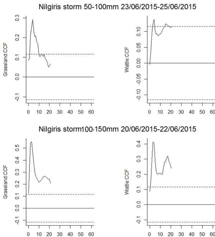
*Figure 4-11: Higher cross-correlation in grassland relative to wattle suggests higher proportion of water from the rainstorm being delivered to the stream by grasslands. The secondary peak in wattle is more pronounced but in both catchments, the initial peak at ~5 hours or less is most likely rapid sub-surface flow but there is indication of deeper ground water contributing to stream flow at ~10-20 hours after the rainstorm.*
