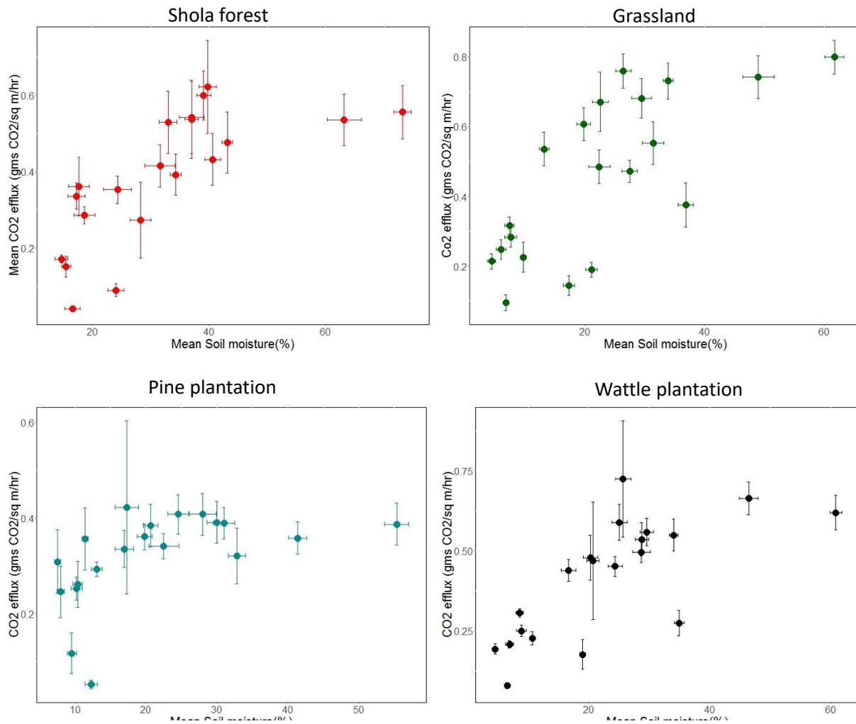
Figure 5-12 Soil CO<sub>2</sub> efflux as a function of soil moisture in (a) shola forests, (b) grasslands, (c) pine plantations and (d) wattle plantations. In general, soil CO<sub>2</sub> efflux rates increased with increasing soil moisture in this system.
