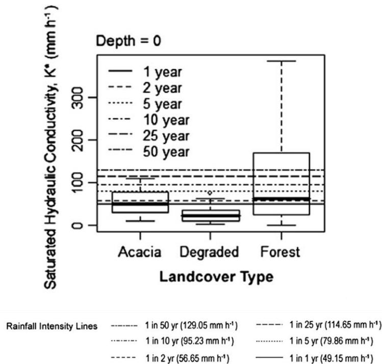
Figure 4-10: Box and Whiskers plots of infiltration rates in top 10 cm of soil under different land-cover with overlay of rain intensity lines in Aghnashini basin, Uttara Kannada. Only the forest soils are able to withstand even the most intense rains without generating infiltration excess overland flow (Adapted from Bonnel et. al 2010)
