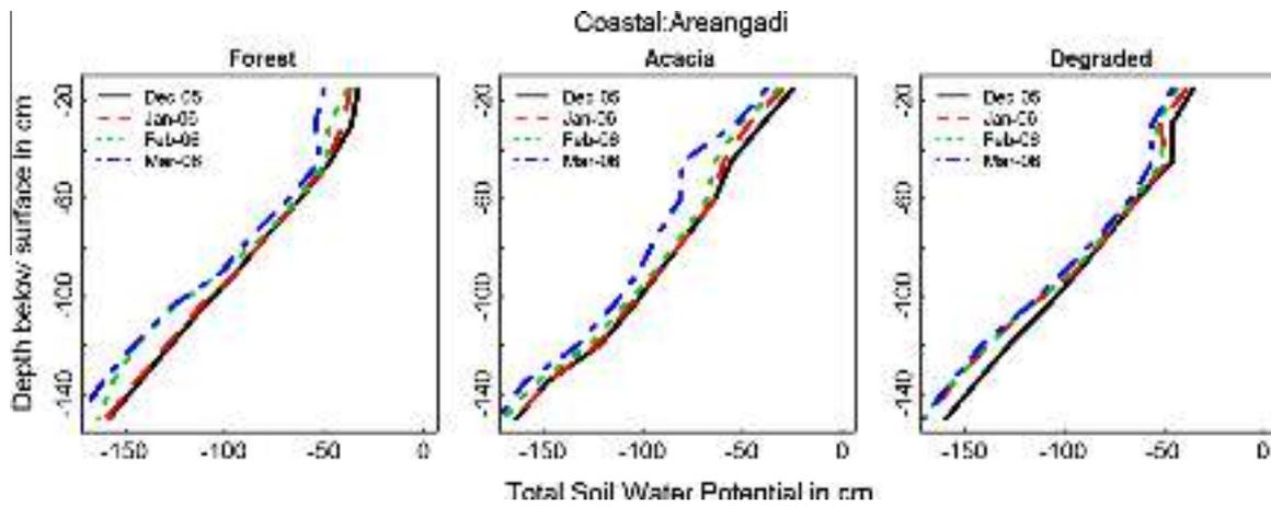
Fig. 7. The total soil water hydraulic potential ( $\Phi$ ) versus depth ( $z$ ) relationsat selected dates during the dry season for the Coastal basins (Sites 1–3, Table 1, Fig. 1), where  $\Phi = \Psi$  (matric potential) –  $z$ (gravitational potential), taking the surface as the reference datum.
