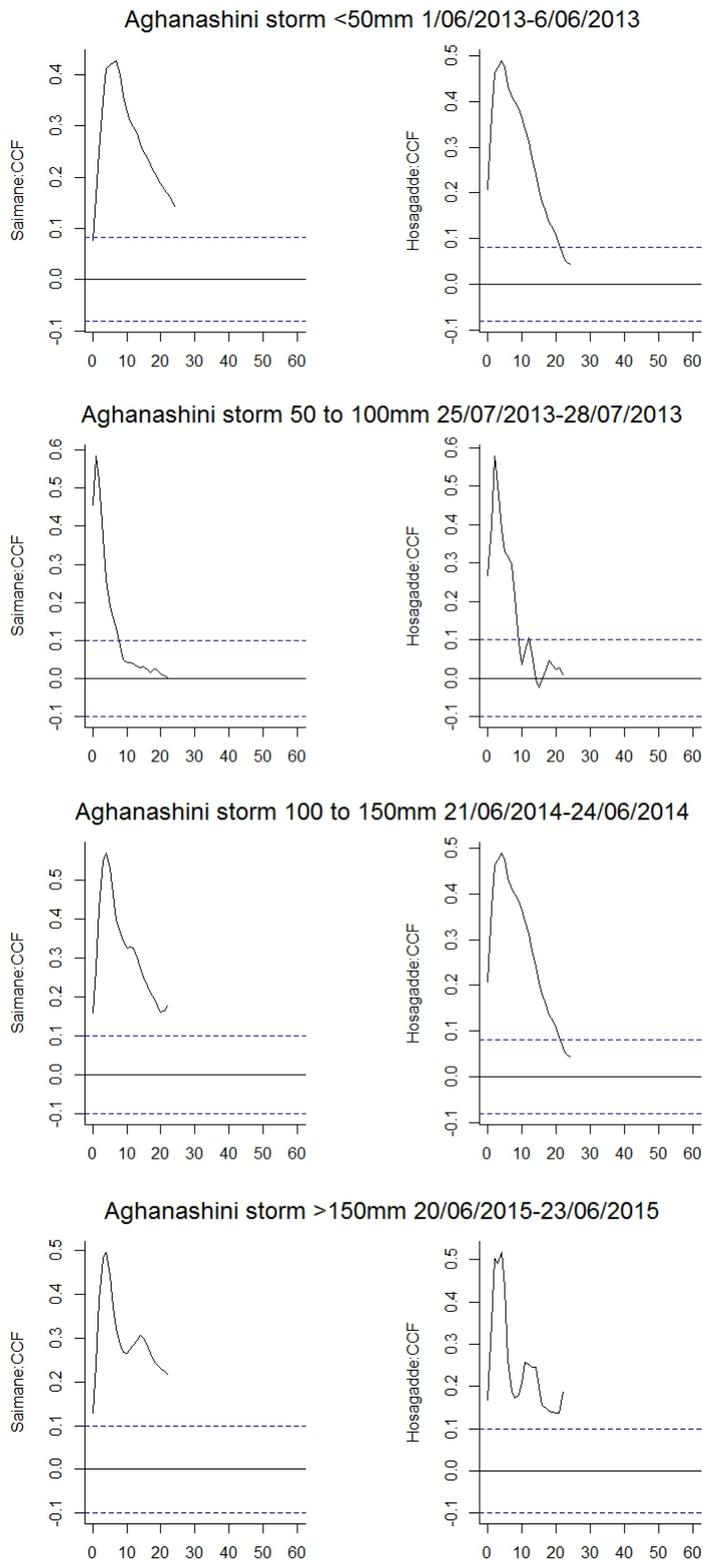
*Figure 4-12: The primary and secondary forest catchments have strong rain water storage capacity in the sub-surface with a primary peak at less than ten hours and a secondary peak being generated in response to the bigger rain storms. Rainstorms totaling over 150 mm per day are likely to generate two flood peaks in these catchments. The primary peak is likely to be generated by shallow rapid sub-surface pathways such as soil pipes.*
