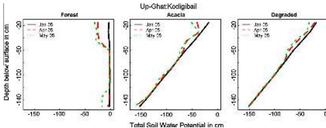
Fig. 8. The total soil water hydraulic potential ( $\Phi$ ) versus depth ( $z$ ) relationsat selected dates during the dry season for the Up-Ghatbasins (Sites 6–9, Table 1, Fig. 1)where  $\Phi = \Psi$  (matric potential) –  $z$  (gravitational potential), taking the surface as the reference datum.
