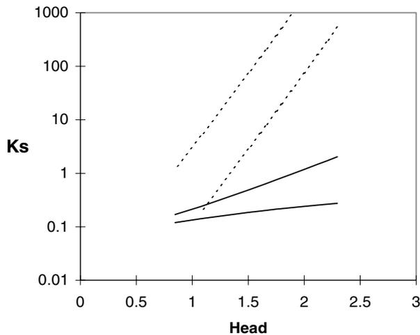
**Figure 31.6** The uncertain band of lateral block permeability derived from the TOPMODEL inversion (between the broken lines,  $K_{SM}$ ) and that derived by up-scaling core-based measurements (between the solid lines,  $K_{SC}$ ). Lateral block permeability has units of  $\times 10^{-6} \text{ m s}^{-1}$  and water-table head is in metres. (After Chappell *et al.*, 1998.)
