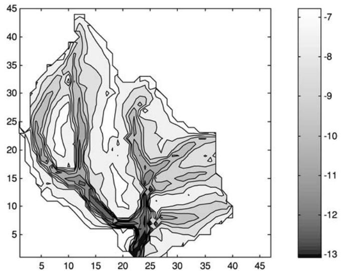
**Figure 31.2** The map of the topographic index ( $\lambda$ ) for the 0.44 km<sup>2</sup> Baru Experimental Catchment, Sabah, Malaysian Borneo. The index ranges from 5.99 to 12.99. The abscissa and y-ordinate axes show the number of grid cells. North is to the top of the figure.
