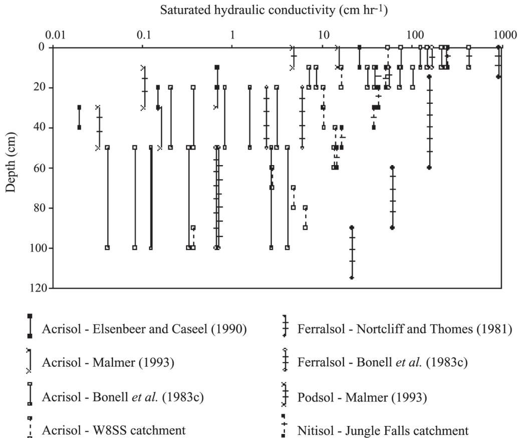
**Figure 31.3** Profiles of saturated hydraulic conductivity (or ‘soil permeability’) from selected tropical soils. The vertical range that each published result represents is shown. (After Sherlock, 1997.)
