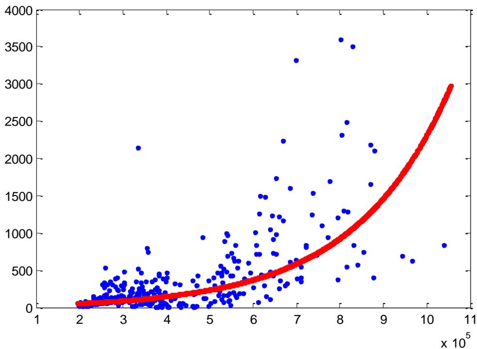
**Fig. 5** The relationship between discharge (x-axis: L s<sup>-1</sup>) and suspended sediment concentration (y-axis: mg L<sup>-1</sup>) for the Sepu gauging station from June 2009 to May 2010 using only a single daily suspended sediment value sampled at noon each day. These data are abstracted from the full 10-minute data-set (Fig. 3).
