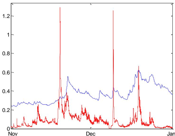
**Fig. 4** The 10-minute sampled load (the time-series with faster dynamics: t<sup>-1</sup>) and discharge (the time-series with more damped dynamics: L s<sup>-1</sup> / 10<sup>6</sup>) data over the first two months of the wet season (i.e., November – December 2009) for the Sepu monitoring station, Upper Ramu drainage basin, Papua New Guinea.
