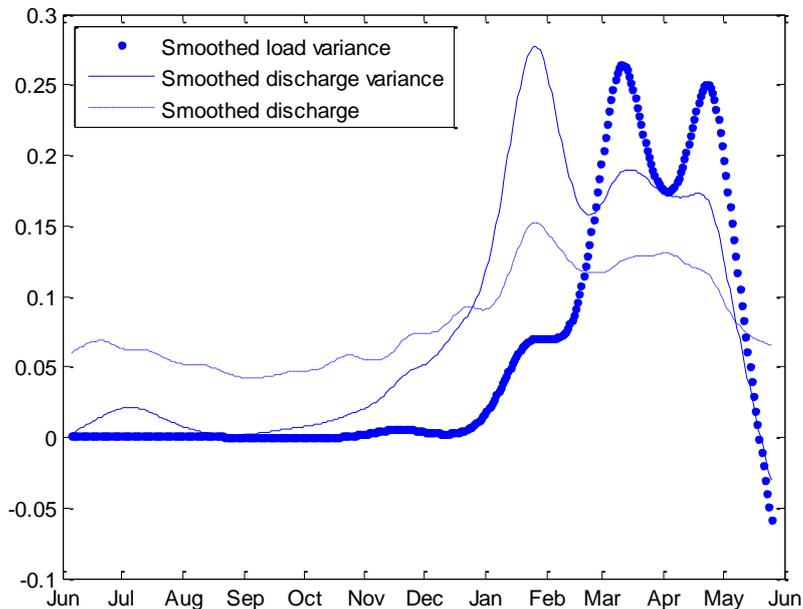
**Fig. 6** Time-series of smoothed variances of suspended sediment load and discharge, plus the smoothed discharge for the Sepu gauging station from June 2009 to May 2010. The discharge variance and mean discharge are scaled by factor of  $2E-11$  and  $2E-7$ , respectively, so that they can be plotted at the same y-axis location as the load variances.
