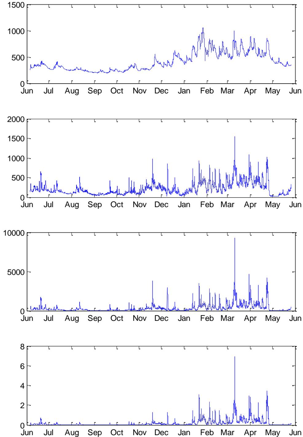
**Fig. 3** The 12-months time series of river discharge ( $\text{m}^3 \text{ s}^{-1}$ ; top), turbidity (NTU; upper middle), suspended sediment concentration ( $\text{mg L}^{-1}$ ; lower middle) and load ( $\text{t s}^{-1}$ ; bottom) recorded every 10 minutes at the Sepu monitoring station ( $5^\circ 27.8' \text{ S}$ ,  $145^\circ 12.6' \text{ E}$ ), Upper Ramu drainage basin, Papua New Guinea.
