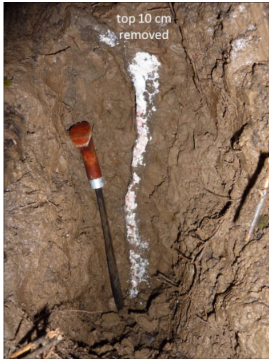
Figure 7. A vertical cicada burrow filled with Plaster of Paris and then excavated (undertaken by V. Grimsey). The shaft extends to a depth of 60 cm (undisturbed soil is observed beneath), and is located only 20 cm from the bank of a gully formed by pipe collapse ( 4^{\circ}57'68''\text{N} , 117^{\circ}48'15''\text{E} ; Figure 3b). The shaft diameter is mostly between 2 and 3 cm. The top 10-cm section of the shaft has been removed and is not visible in the photograph
