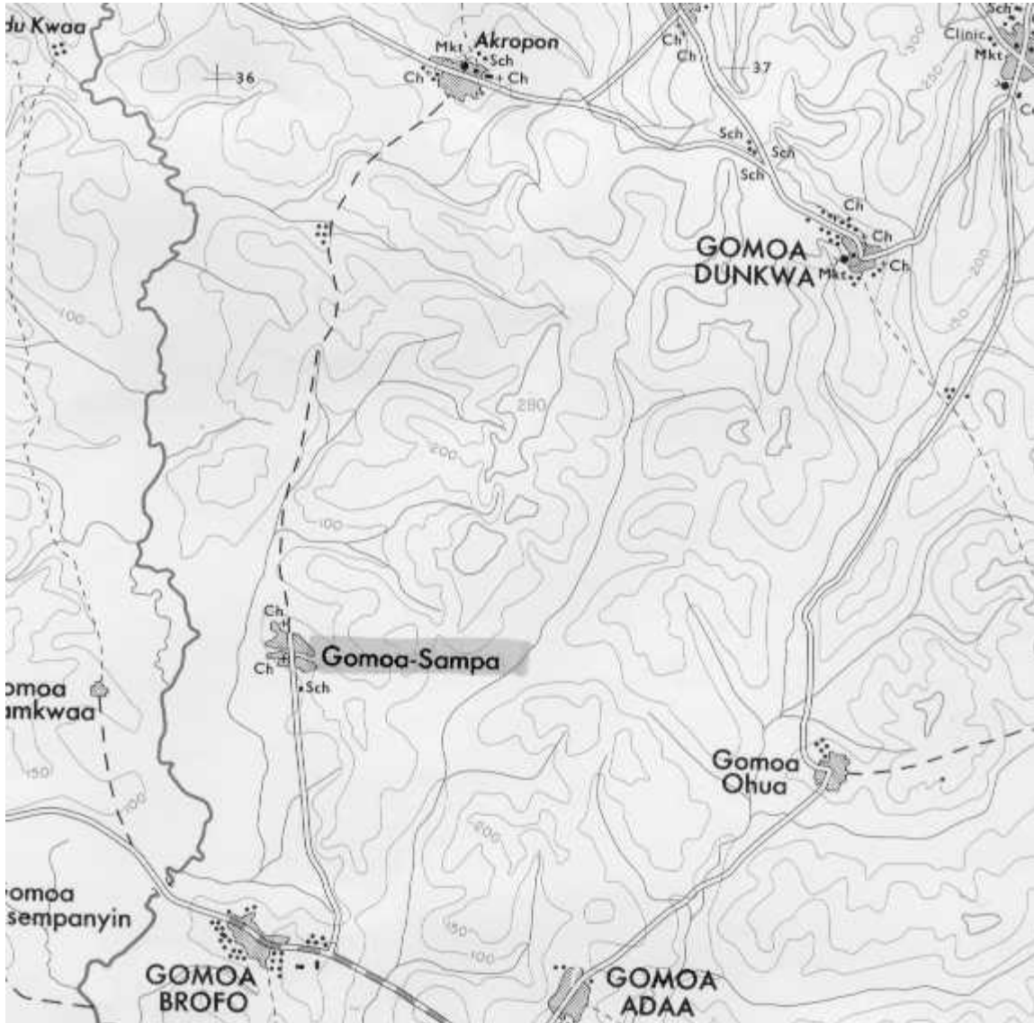
Figure 16. Regional feeder roads (=), topography (-) and some paths (- -) in the vicinity of Sampa village. Note that the feeder road from Sampa to Akropon is only shown as a path on this old map. Adapted from map sheet 0501C1 (1:50,000 scale), Survey of Ghana.
