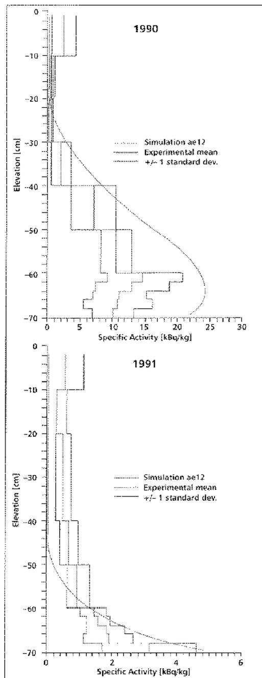
**Figure 16** Observed and predicted distribution of  $^{22}\text{Na}$  in a column experiment conducted in the laboratory
