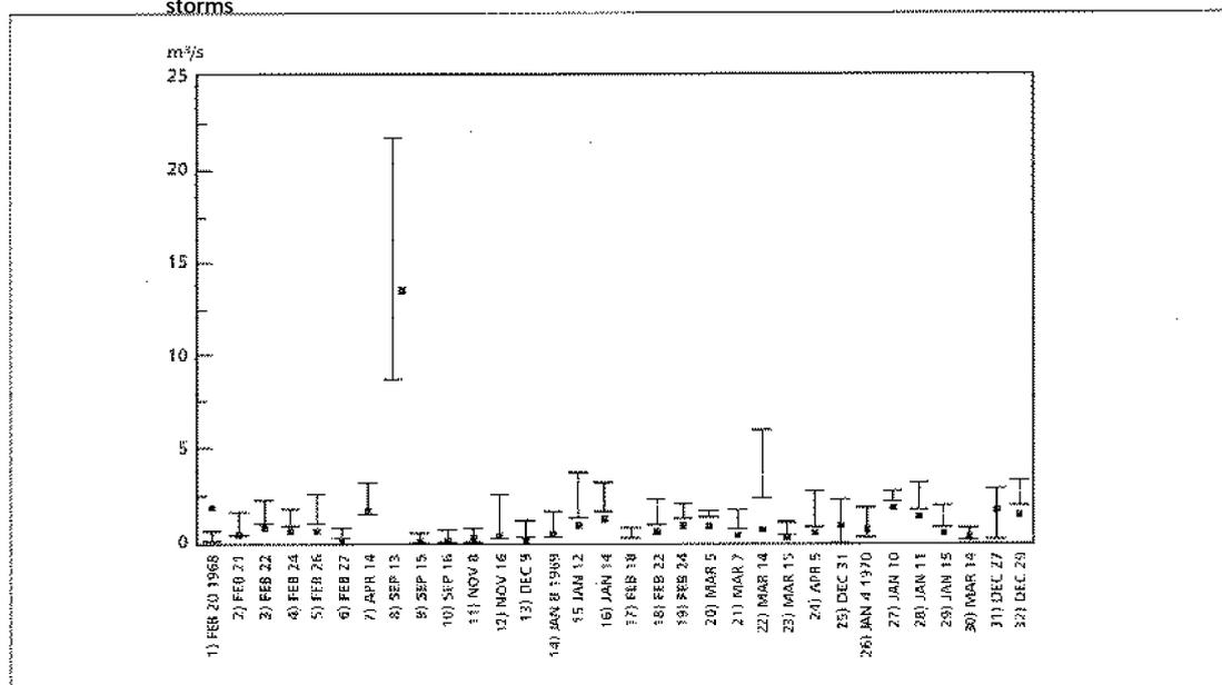
Figure 9 Validation of SHETRAN-UK for the Rimbauld catchment: Test C - monthly discharge during wet months
