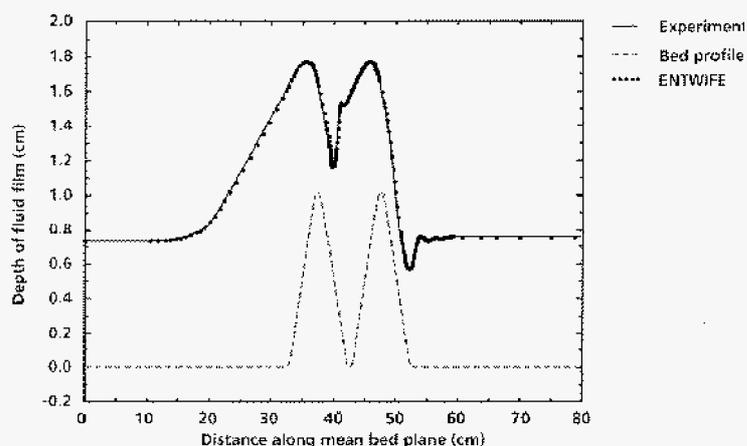
**Figure A: Comparison of ENTWIFE computation with laboratory experiment for flow of a viscous fluid down a perturbed inclined plain. The depth of the fluid film is plotted against distance along the plain.**
