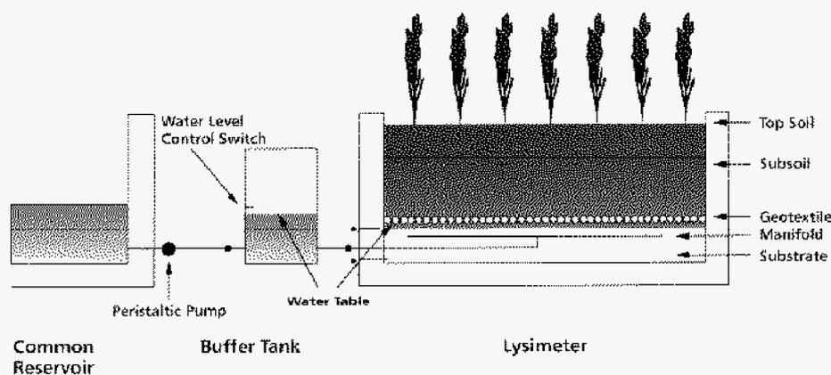
Figure A: Water level control in the phase 1 lysimeters (not to scale).
