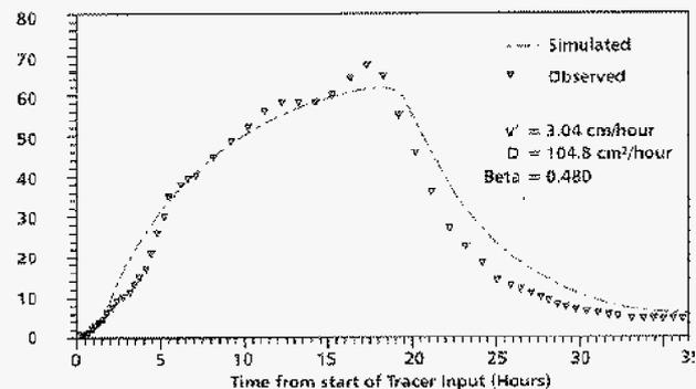
Figure B: Fitted breakthrough curve for return flow through a large undisturbed soil core. Note the very rapid initial breakthrough and long tail indicative of preferential flow in macropore pathways and a very high dispersion coefficient.
